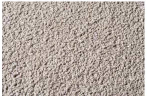
Closed corundum-gritted surface (KB) – slip resistant R13
