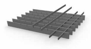
Press-locked grating is frequently used in outdoor applications or other areas where there is a particularly high requirement for the slip-resistant properties of the floor covering. The grating can be manufactured with a slip resistance class of R10 to R13 and because many different mesh spacings can be manufactured, drop-through protection for various small parts can be guaranteed whilst ensuring compatibility with fire sprinkler systems for levels located below.
