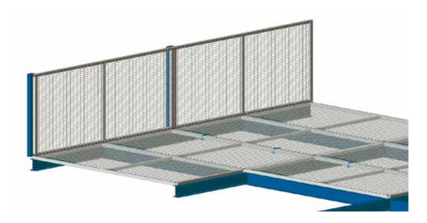
A distinction is made with respect to the fall protection panels between floor elements & side protection.
