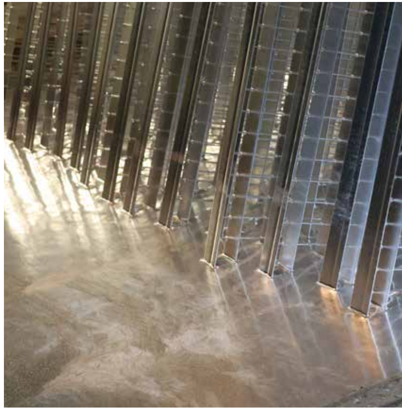
Batch galvanising also reaches hard-to-access areas, ensuring continuous protection across the entire surface
