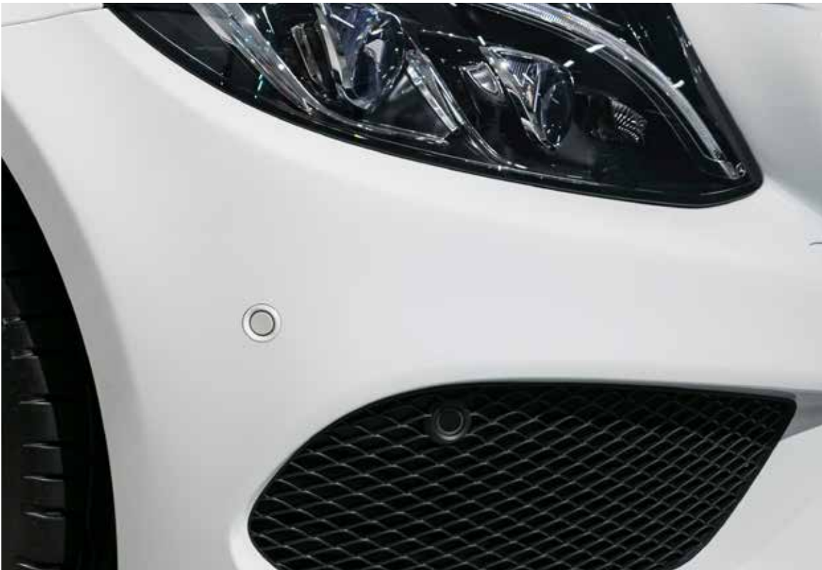
Expanded metal is used in modern vehicles and impresses with stability and low weight
