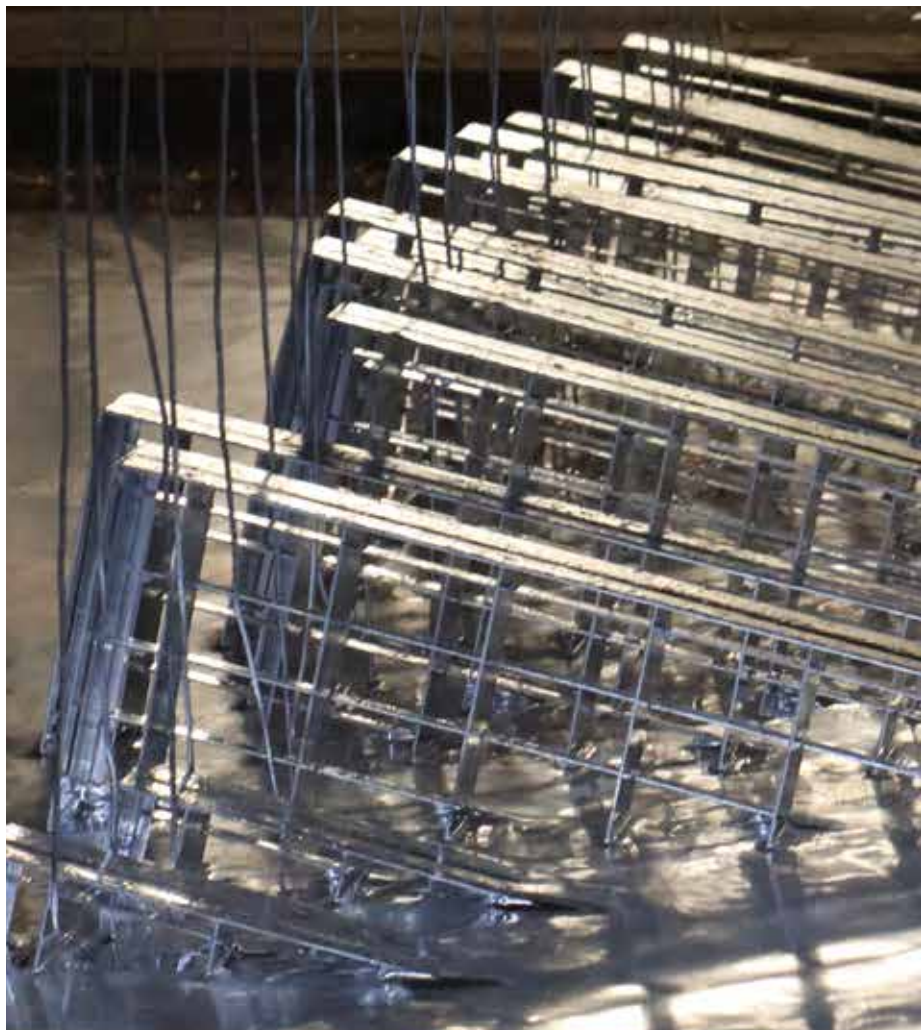
Batch galvanising provides lasting protection against corrosion, ensuring robust, low-maintenance use outdoors
