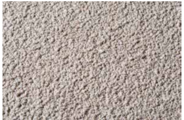
Closed corundum-gritted surface (KB) – slip resistant R13
